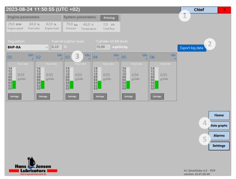
The main Home screen offers a broad overview of the system and provides easy access to various features such as graphs, alarms and settings. Engine and system parameters are also visible at the top of the screen.
