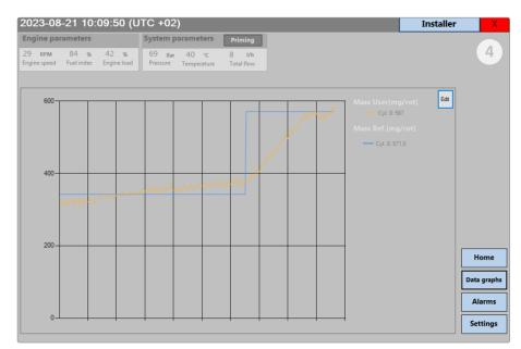
The Data Graphs screen shows reference consumption (blue line) and actual lube oil consumption. Edit the graph by selecting the cylinders you want to see for comparing performance.
