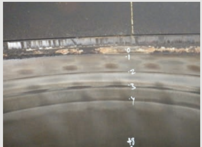
Cylinder 8 equipped with standard electronic lubrication - wave cuts not visible.
