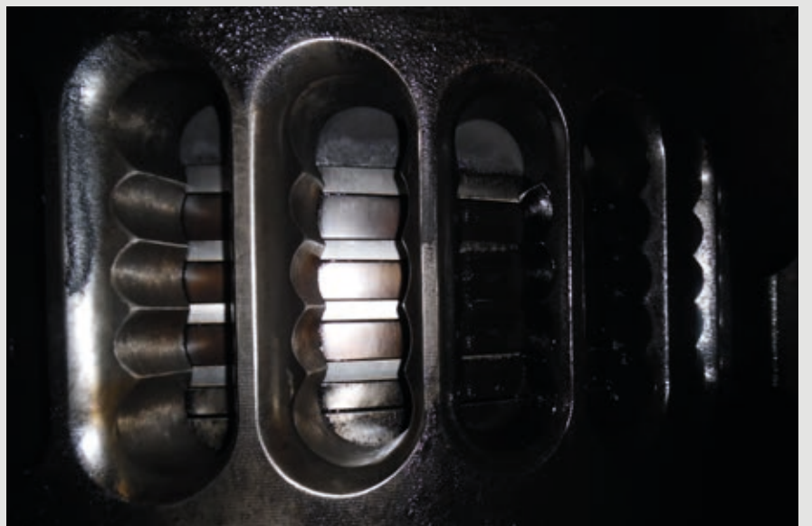
Half cleaned – smooth piston rings.
