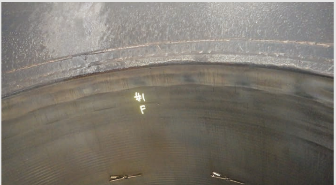
Cylinder 1 equipped with HJ Lubtronic SIP - wave cuts still visible.
