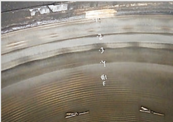
Cylinder 1 equipped with HJ Lubtronic SIP - wave cuts still visible.
